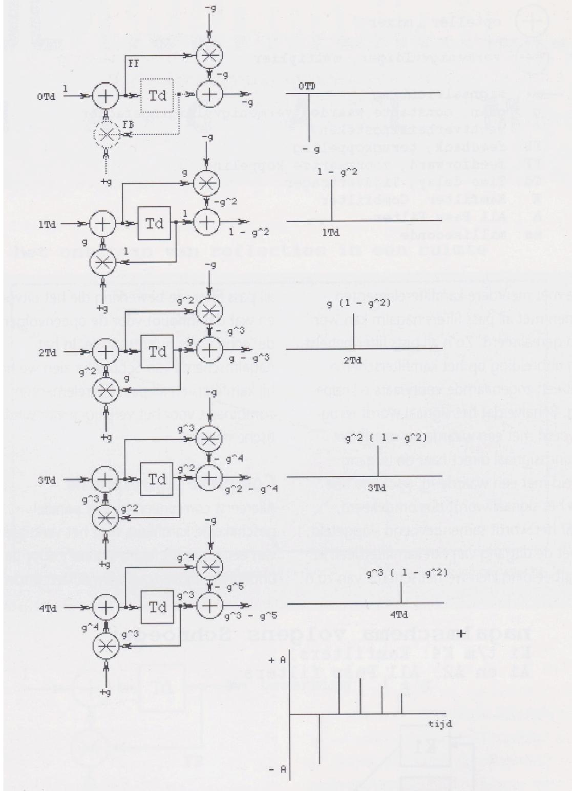
Such a pulse response description is the counterpart of the operation in the frequency domain, the frequency characteristic, which in principle amounts to the same thing. The realization at the bottom left of the image is the way Schroeder realized his allpass network, which
