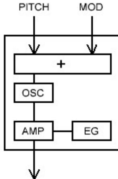
Each operator, both carrier and modulator comprises an input mixer where pitch data PITCH, the keys, and modulation data MOD, are mixed. The mixer output is now the control input of the oscillator OSC. By means of the envelope generator, EG, the amplitude of the oscillator can be controlled dynamically in the AMP.
