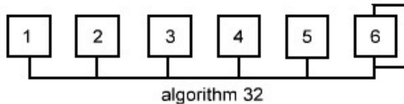
In this configuration we see all six operators coexist. Their outputs are simply added together (mixed). In this example, we basically obtain the additive synthesis model. Additive means literally add, mixing. All operators now function as carriers. Modulators are missing here completely.
